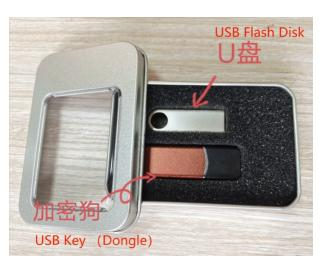
9.1 Turn-on software if appear"can't find key lock".this, means that you didn't plug into software, or computer USB port doesn't touch good, you need to change another port to plug into.
